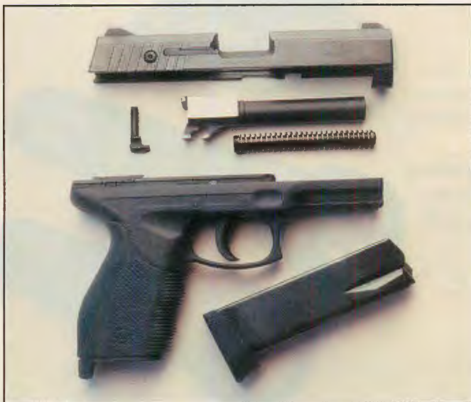
The 24/7 can be field stripped as shown in about a minute or less. Reassembly is about as fast.
